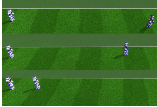
Figure 2.11: The top panel shows the distance covered by the agent after optimization. The middle panel shows the distance covered by our hand-tuned solution. The bottom panel shows the stable initial hand-tuned solution given to CREPS-CMA.
